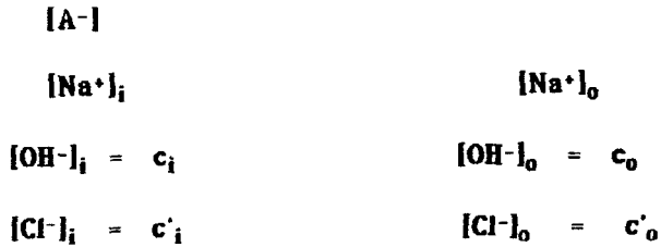
FIGURE 1. Distribution of an aqueous solution containing NaOH and NaCl between inner and outer solutions of a gel containing fully ionized acidic groups A^- . Subscripts i and o signify inner and outer solutions, respectively.
